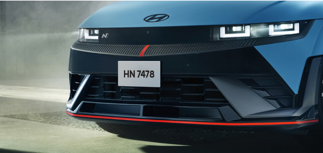
N-exclusive Front Bumper with Active Air Flaps and Air Curtains
