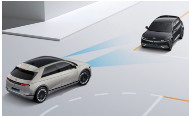
Forward Collision-Avoidance Assist (FCA)*
